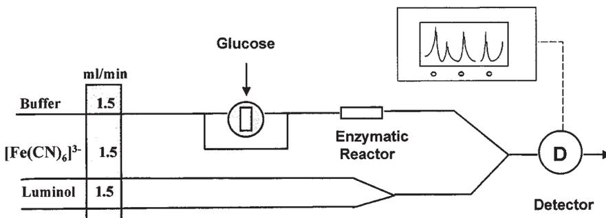
Figure 7. Schematic diagram for a FIA manifold for the analysis of glucose incorporating an enzymatic reactor with detection based on the luminol reaction.
