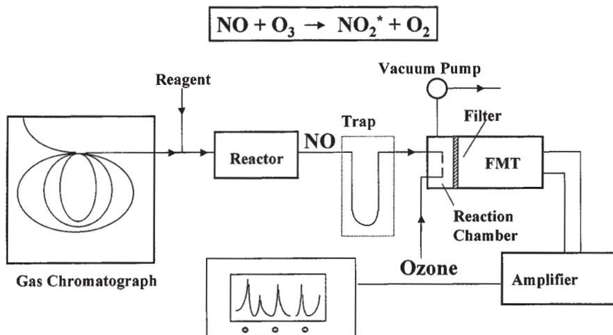
Figure 6. Schematic diagram for CL detection in gas chromatography.
