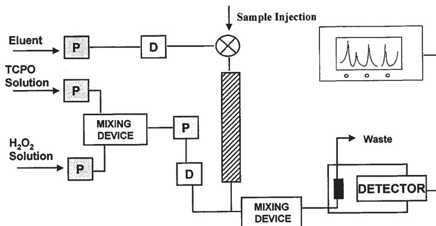
Figure 8. Schematic diagram for a post-column CL-based detection system used in HPLC (D, damper; F, flow-cell; I, injector; MC, mixing coil; P, pump; PM, photomultiplier tube; R, recorder).
