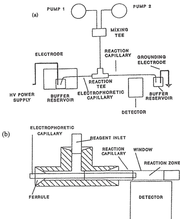
Figure 9. Example of a CE-CL system. (a) Experimental configuration. The hydrogen peroxide is introduced by pump 1 and pump 2 provides base. (b) Cross sectional scheme of the CL detection interface (with permission from réf. [120]).
