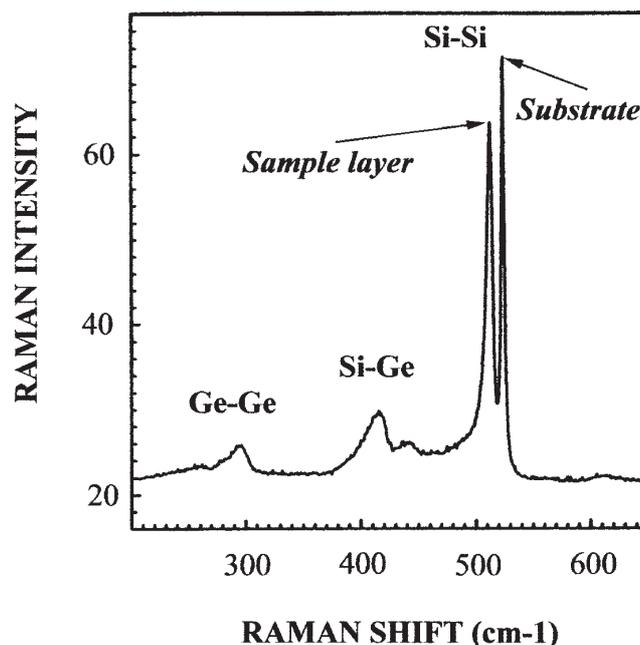
Figure 1. Raman spectrum of  $\text{SiGe}_{0.3}$ , showing the Si-Si, Ge-Ge and Si-Ge vibrational modes. The Raman band at  $520\text{ cm}^{-1}$  is due to the crystalline Si substrate.
