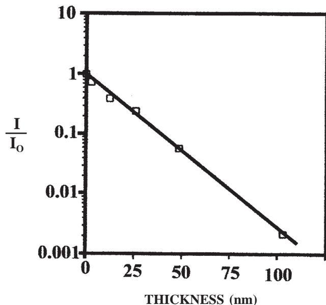
Figure 4. Relative Raman intensity of the first order Si mode in function of  $\text{CoSi}_2$  thickness.
