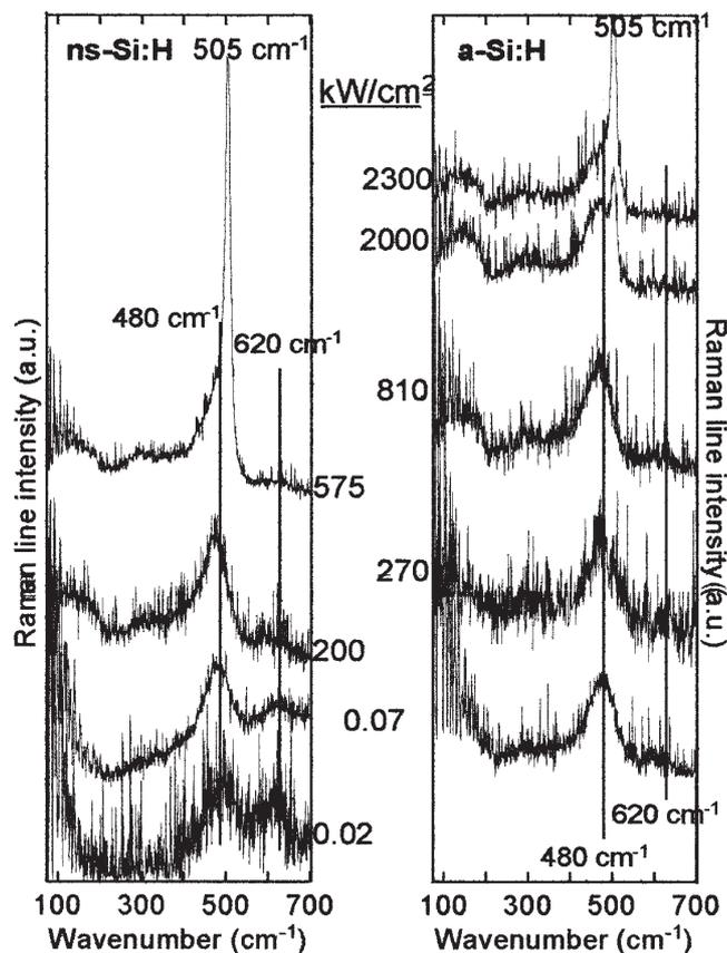
Figure 7. *In situ* evolution of the Raman spectrum of hydrogenated nanostructured silicon (ns-Si:H) and hydrogenated amorphous silicon (a-Si:H) thin films with the laser power density (Courtesy of G. Viera).
