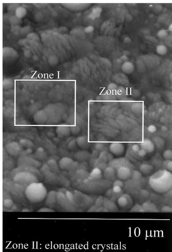
Figure 8. Micro-Raman spectra recorded in two different zones of a calcium-phosphate coating deposited by laser ablation with the corresponding SEM micrograph indicating the respective regions (Courtesy of L. Cléries).
