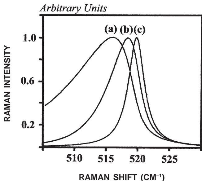
Figure 2. Simulation of the silicon first order Raman phonon mode assuming spherical confinement: (a)  $L = 60 \text{ \AA}$ , (b)  $L = 100 \text{ \AA}$ , (c)  $L = 200 \text{ \AA}$ .
