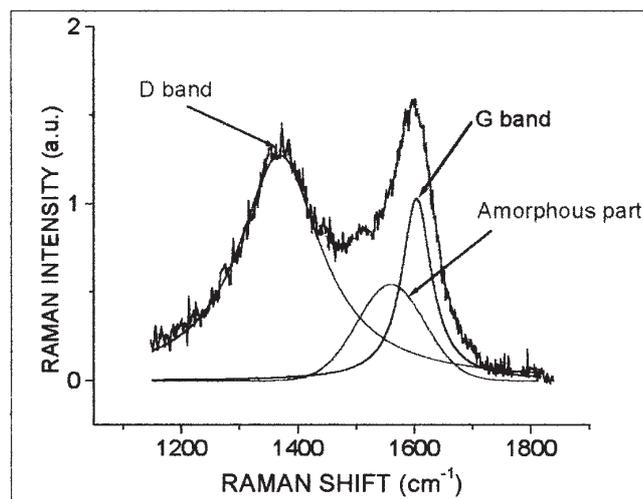
Figure 5. Micro-Raman spectrum of a single particle of black carbon with the corresponding curve fitted bands.
