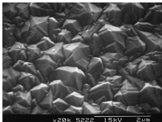
Figure 6(a). AFM micrograph of some precursor crystals with the Raman spectrum of one of these crystallites (Courtesy of M.C. Polo).
