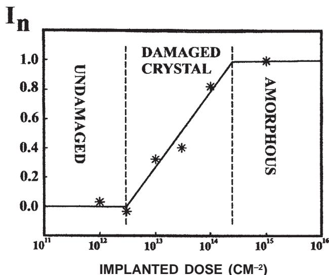
Figure 3. Relative micro-Raman intensity of the Longitudinal Optical mode of 6H-SiC versus the implantation dose.
