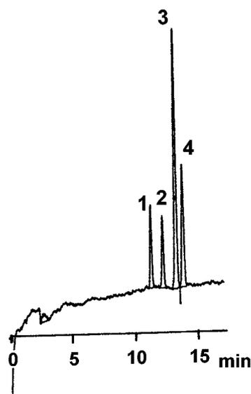
Figure 2. Electrochromatographic separation on a soft gel column. Conditions: column, 0.075 mm i.d.  $\times$  48.5 cm (active length, 24.0 cm); stationary phase, 4.1%T, 9.7%C, .7%S poly(AMPS-co-IPAAm); mobile phase, 20:80 v/v mixture of acetonitrile and 2.5 mM phosphate buffer (pH 6.8); voltage, 16 kV. Peaks: benzyl alcohol (1), resorcinol (2), methylparaben (3) and  $\beta$ -naphthol
