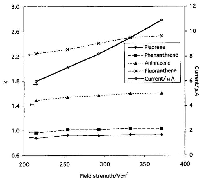
Figure 3. The retention factor,  $k$ , of polycyclic aromatic hydrocarbons on a 7.7%T, 3.9%C, 9.4%S poly(AMPS-co-4-acryloylmorpholine-co-allyl *n*-octyl ether) column as a function of the field strength. Conditions: column, 0.050 mm i.d.  $\times$  51.2 cm (active length, 25.2 cm); mobile phase, 20:80 v/v mixture of acetonitrile and 0.10 M Tris-0.15 M boric acid buffer (pH 8.2).
