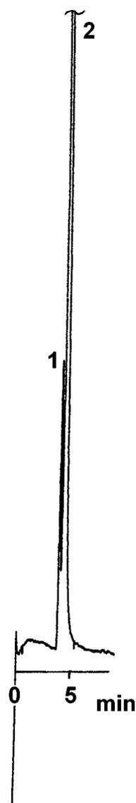
Figure 1. Electrochromatographic separation on a particle-fused column. Conditions: column, 0.150 mm i.d. × 37.0 cm (active length, 20.0 cm); mobile phase, 20:80 v/v mixture of acetonitrile and 2.5 mM phosphate buffer pH 6.8; voltage, 15 kV. Peaks: naphthalene (1) and phenanthrene (2).
