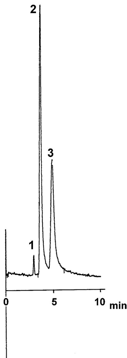
**Figure 4.** Electrochromatographic separation on a sol-gel-derived column. Conditions: column, 0.075 mm i.d.  $\times$  50.5 cm (active length, 26.0 cm); stationary phase, 4.1%T, 9.7%C, .7%S poly(AMPS-co-IPAAm); mobile phase, 20:80 v/v mixture of acetonitrile and 2.5 mM phosphate buffer (pH 6.8); voltage, 20 kV. Peaks: acetone (1), acetophenone (2), and propiophenone (3).
